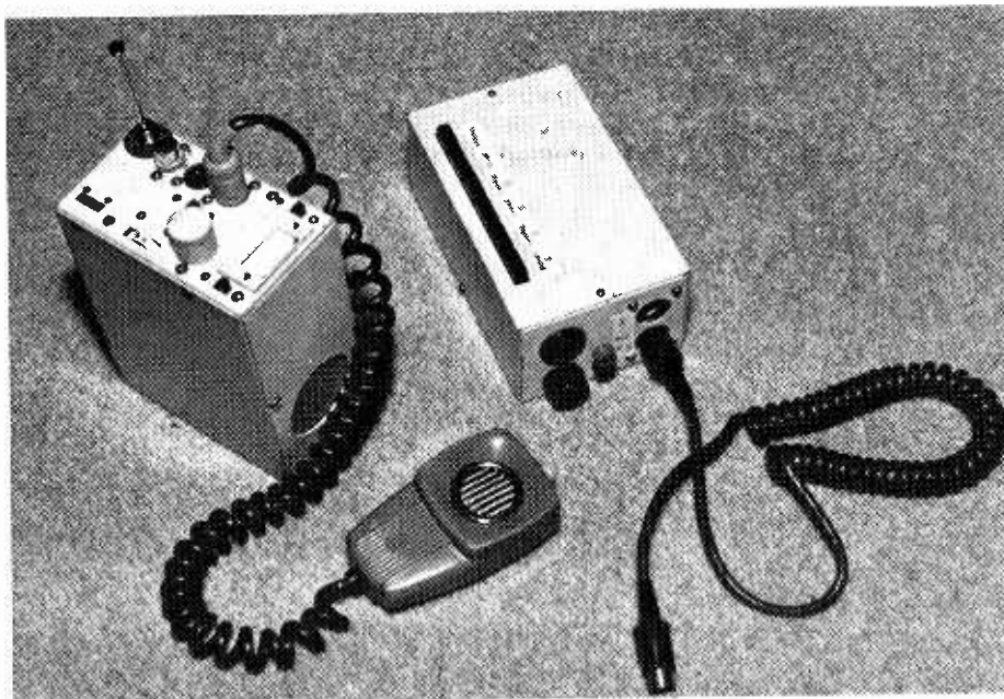
The transceiver and its main power unit and battery charger.
