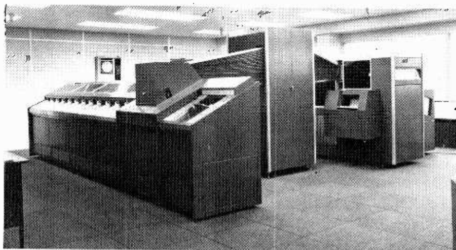
Character reading system with electronic retina in tall central cabinet. On the left is a document carrier, and on the right a page carrier. The concertina-like structures shroud the character image from extraneous light.
